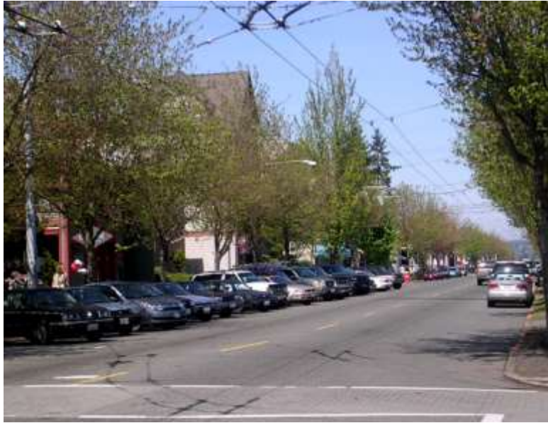
Back-in angle parking allows for a safer, more efficient use of space in Dayton
