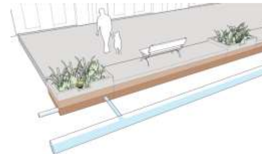
Figure 2.3 NACTO Example of Flow Through Planter Source: NACTO Urban Street Design Guide (2013)
