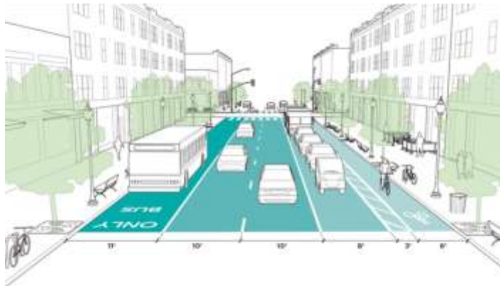
Figure 2.11 After Redesign Using 10-ft Lanes with bike lane Source: NACTO Urban Street Design Guide (2013)
